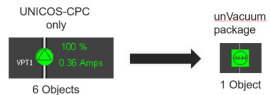
Figure 1: Turbomolecular pump widget without and with the vacuum package.
