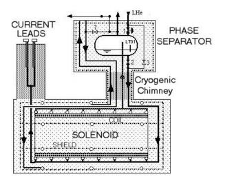
Fig. 2 The Coil Cryogenic System
