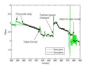
Fig. 8 Pressure in the coldbox phase separator during unusual operation
