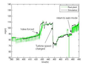
Fig. 9 mass flow of turbine 1 during unusual operation
