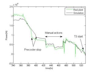
Fig. 11 Energy balance of the Coil Cryogenic System
