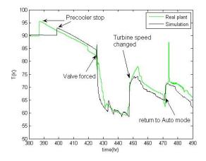
Fig. 7 Temperature after the first heat exchanger during unusual operation
