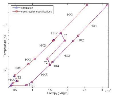
Fig. 13 T-S diagram of the coldbox at 4.5K
